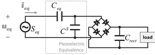
Fig. 3. Equivalent circuit for standard energy harvesting.
