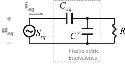
Fig. 4. Equivalent circuit for resistive shunt damping.
