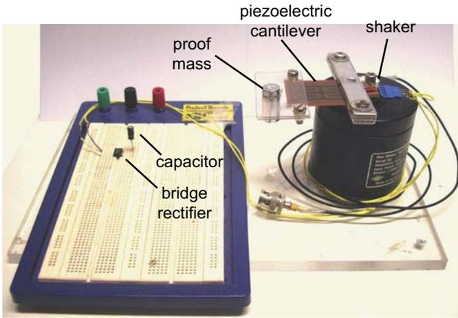
Fig. 7. Experimental setup for standard energy harvesting.
