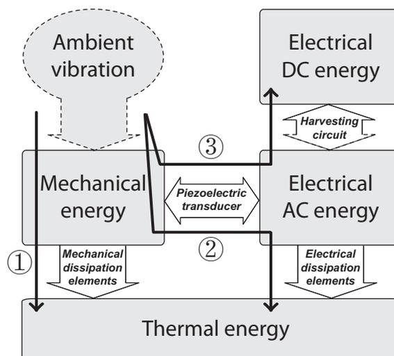
Fig. 1. Energy flow chart in piezoelectric devices.
