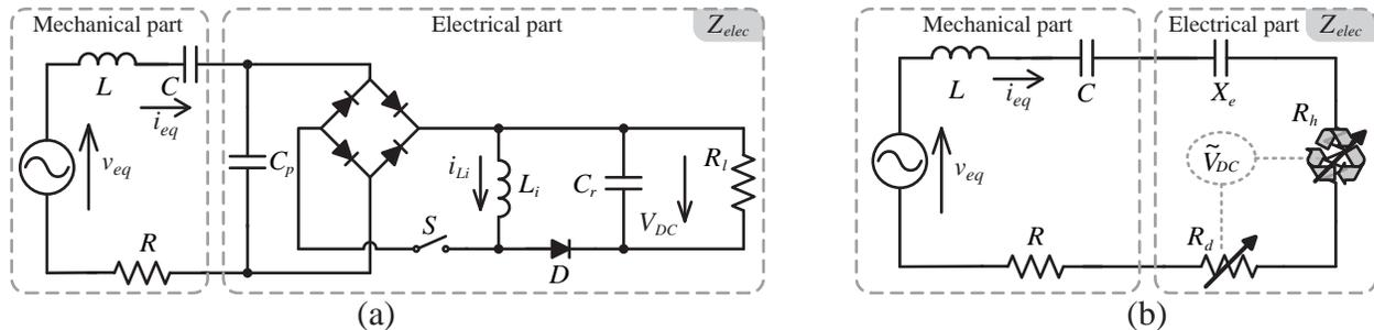
Figure 2. (a) Equivalent circuit. (b) Equivalent impedance network.
