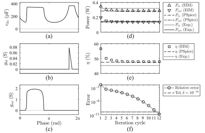
Fig. 6. Results with sinusoidal gate-drive voltage. (a) Nonlinear junction capacitance  $c_{ds}$ . (b) Body diode conductance  $g_{bd}$ . (c) Switch conductance  $g_{sw}$ . (d) Input and output powers. (e) Conversion efficiency. (f) Relative errors in iteration.
