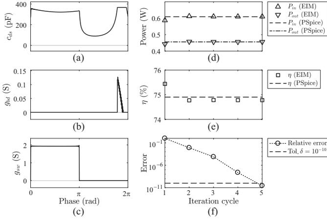
Fig. 5. Results with square-wave gate-drive voltage. (a) Nonlinear junction capacitance  $c_{ds}$ . (b) Body diode conductance  $g_{bd}$ . (c) Switch conductance  $g_{sw}$ . (d) Input and output powers. (e) Conversion efficiency. (f) Relative errors in iteration.
