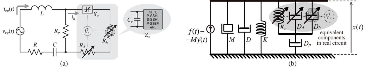
Figure 2. The electrical and mechanical equivalent models of a PEH system using practical single-variable tunable harvesting circuits.<sup>12</sup> (a) The equivalent impedance model. (b) The responding equivalent mechanical schematic.
