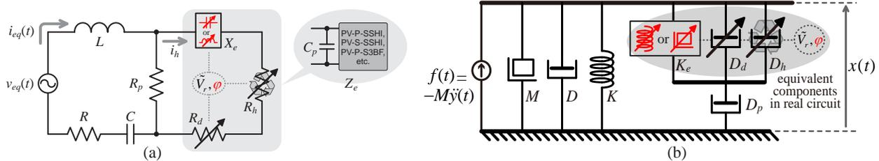
Figure 3. The electrical and mechanical equivalent models of a PEH system using practical double-variable tunable harvesting circuits. (a) The equivalent impedance model. (b) The responding equivalent mechanical schematic.
