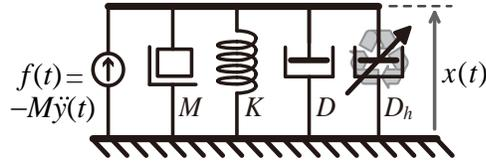
Figure 1. The early conceptual schematic model of a kinetic energy harvester.<sup>11</sup>
