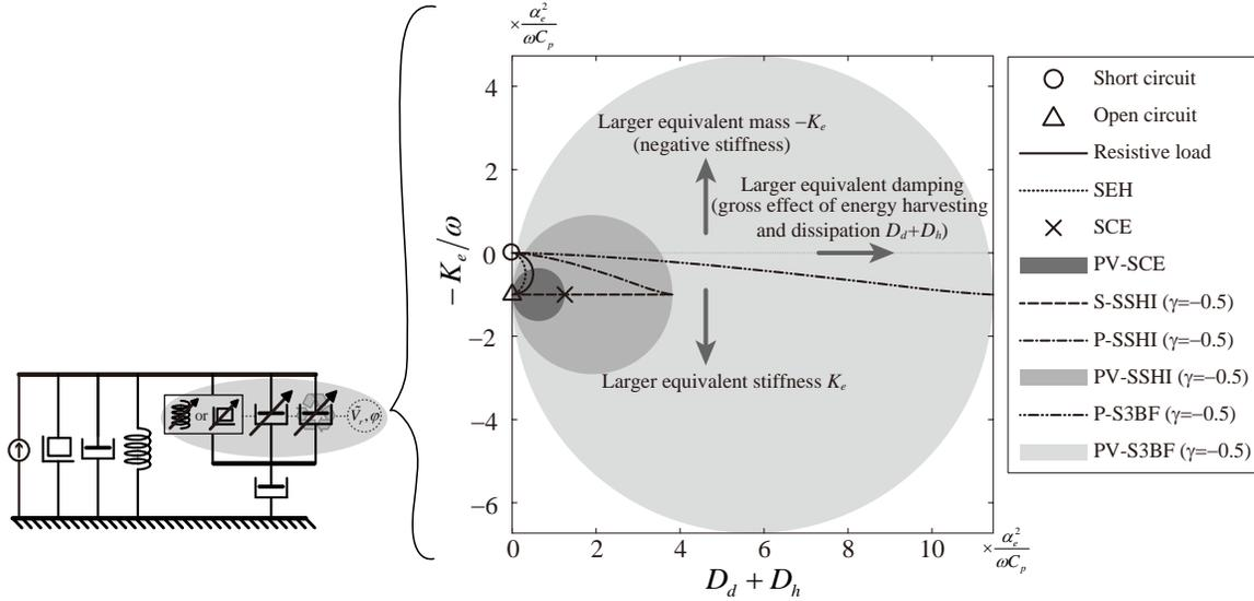
Figure 4. The attainable ranges of the electrically induced mechanical dynamics of different PEH interface circuits.
