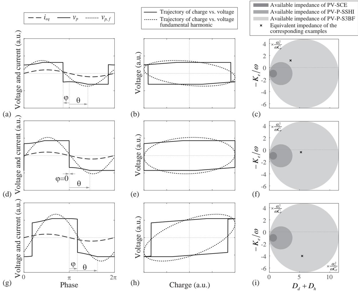
Figure 5. Waveforms and impedance pictures of PV-P-S3BF under different switching phase lag  $\varphi$  ( $\gamma = -0.5$ ). (a)-(c) Phase lead switch. (d)-(f) In phase switch. (g)-(i) Phase lag switch. (a), (d), and (g) Voltage and current waveforms. (b), (e), and (h) The original work cycles and their linear approximations. (c), (f), and (i) The corresponding equivalent impedances in the impedance plane.
