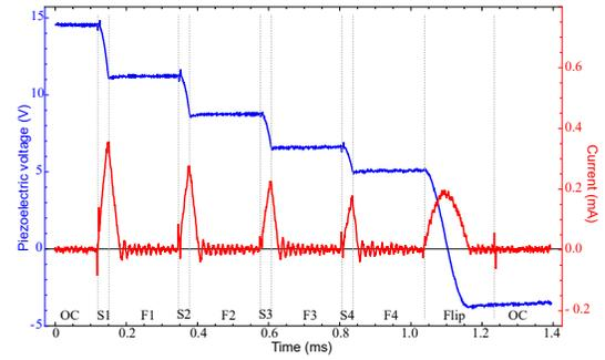
Fig. 7. Experimental piezoelectric voltage and inductor current waveform at a downstairs synchronized instant.
