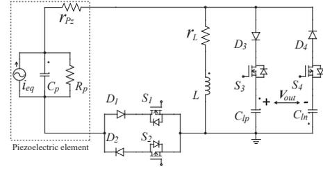
Fig. 2. Simplified schematic of MCEBF circuit
