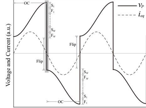
Fig. 3. Operating waveform of MCEBF circuit
