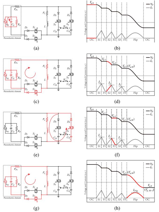
Fig. 4. Operating phases in the falling edge. (a)(c)(e)(g) Conduction branches. (b)(d)(f)(h) Waveforms of the piezoelectric voltage and inductor current. (a)(b) Open-circuit phase. (c)(d) One of the Switching phases. (e)(f) One of the Freewheeling phases. (g)(h) Bias-flipping phase.
