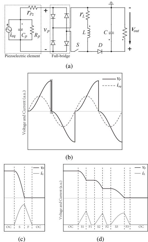
Fig. 1. Topology and waveforms of SECE and MCE interface circuit. (a) Typical topology of SECE interface circuit. (b) Piezoelectric voltage and equivalent current waveforms. (c) Enlarged view of a synchronized switch instant in SECE. (d) Enlarged view of a synchronized switch instant in 3CE
