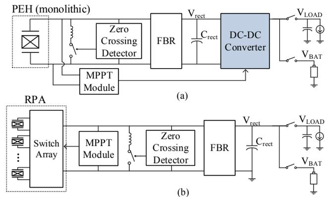
Fig. 1. (a) Conventional PEH system, (b) PEH system based on RPA and the P-SSHI rectifier
