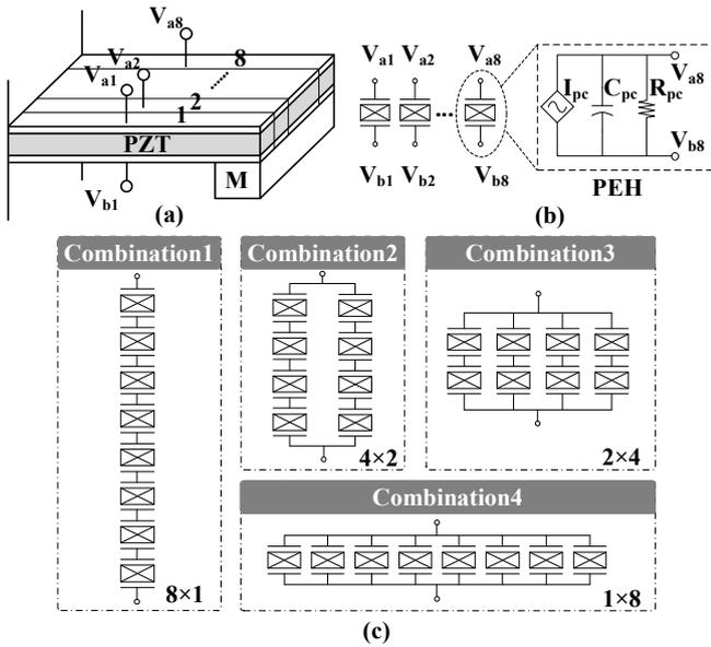
Fig. 2. Representation of RPA: (a) physical structure, (b) equivalent electrical model and symbol, (c) proposed configurations.
