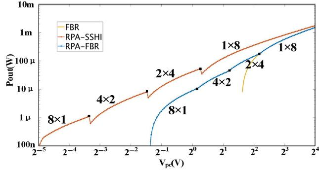
Fig. 9. Output power of FBR, RPA-FBR and the proposed RPA-SSHI
