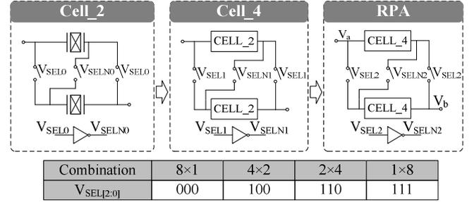
Fig. 4. Hierarchical structure implementation of the proposed RPA
