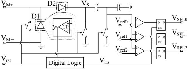
Fig. 5. Structure of MPPT module
