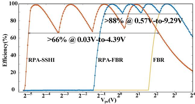
Fig. 8. Power conversion efficiency of FBR, RPA-FBR and the proposed RPA-SSHI
