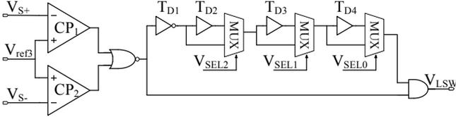
Fig. 6. Structure of proposed RPA based zero-crossing detector
