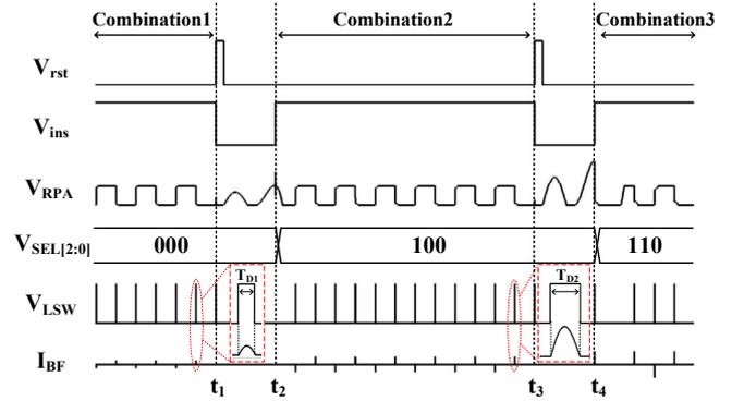
Fig. 7. Simulated waveform of the system control signals
