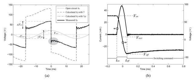
**Figure 4.** Characteristic waveforms in s-SSHI ( $V_{OC} = 20$  volt,  $V_{rect} = 7.6$  volt). (a) Voltages. (b) Zoom-in view to the voltage and current around time origin.
