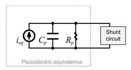
**Figure 5.** Revised equivalent circuit of a piezoelectric device.
