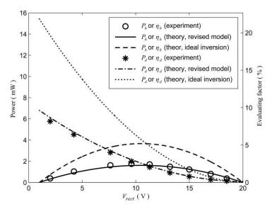
Figure 8. Power and evaluating factors in PEH with s-SSHI interface.
