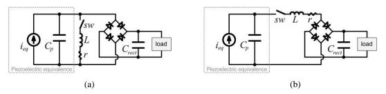
Figure 2. Equivalent circuits of two SSHI treatments. (a) p-SSHI. (b) s-SSHI.
