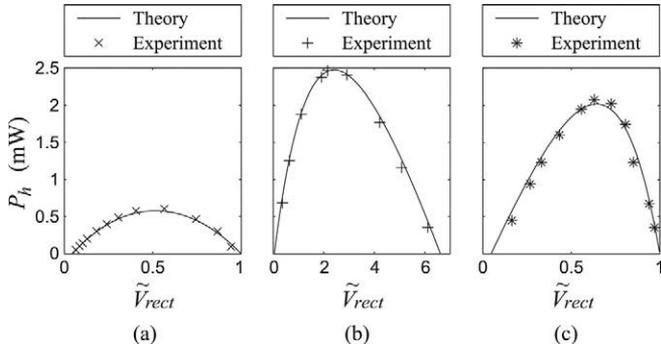
Fig. 14. Theoretical and experimental results on the harvested power with different interface circuits. (a) SEH. (b) P-SSHI. (c) S-SSHI.
