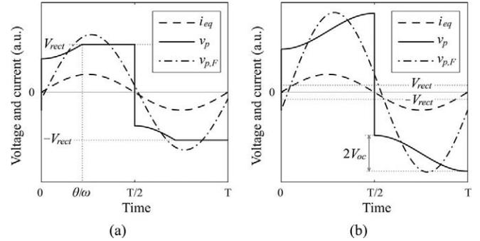
Fig. 5. Characteristic voltage and current waveforms in the SSHI interface circuits. (a) P-SSHI. (b) S-SSHI.
