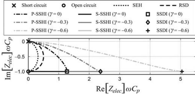
Fig. 6. Electrical part equivalent impedance with four different interface circuits (nondimensionalized with  $(\omega C_p)^{-1}$ , the impedance magnitude under open circuit condition).
