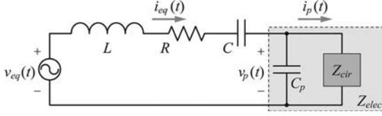
Fig. 2. Equivalent circuit of a base excited PEH device.
