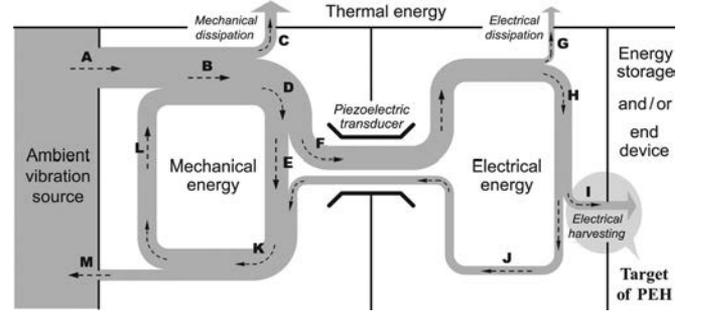
Fig. 7. Energy flow chart of a base excited PEH device.
