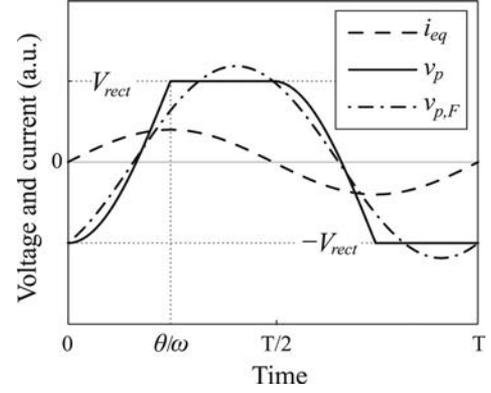
Fig. 3. Characteristic voltage and current waveforms in SEH.
