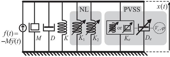
FIG. 3. Equivalent lumped-parameter model of a dual-effect NL-PVSS-PEH system.
