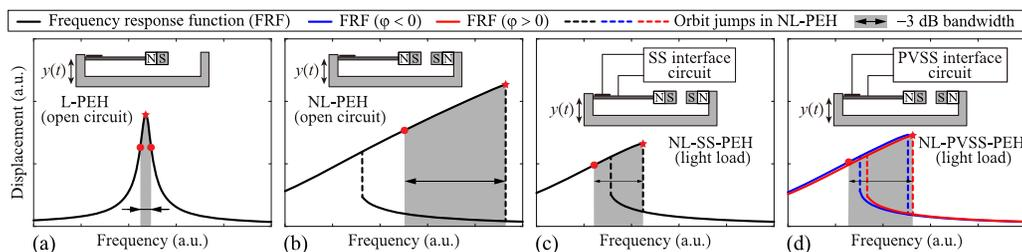
**FIG. 2.** Conceptual development from linear PEH to nonlinear PVSS PEH systems. Sub-figures show the schematics and frequency responses of (a) linear PEH system, (b) nonlinear PEH system, (c) nonlinear PEH system using the SS circuit, and (d) nonlinear PEH system using the PVSS circuit.
