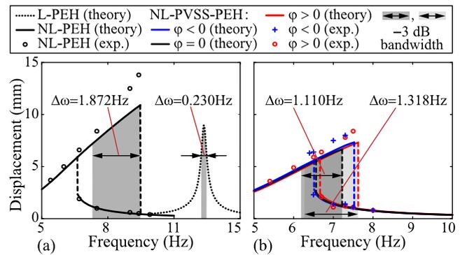
FIG. 5. Theoretical and experimental results. (a) L-PEH and NL-PEH. (b) NL-PVSS-PEH.
