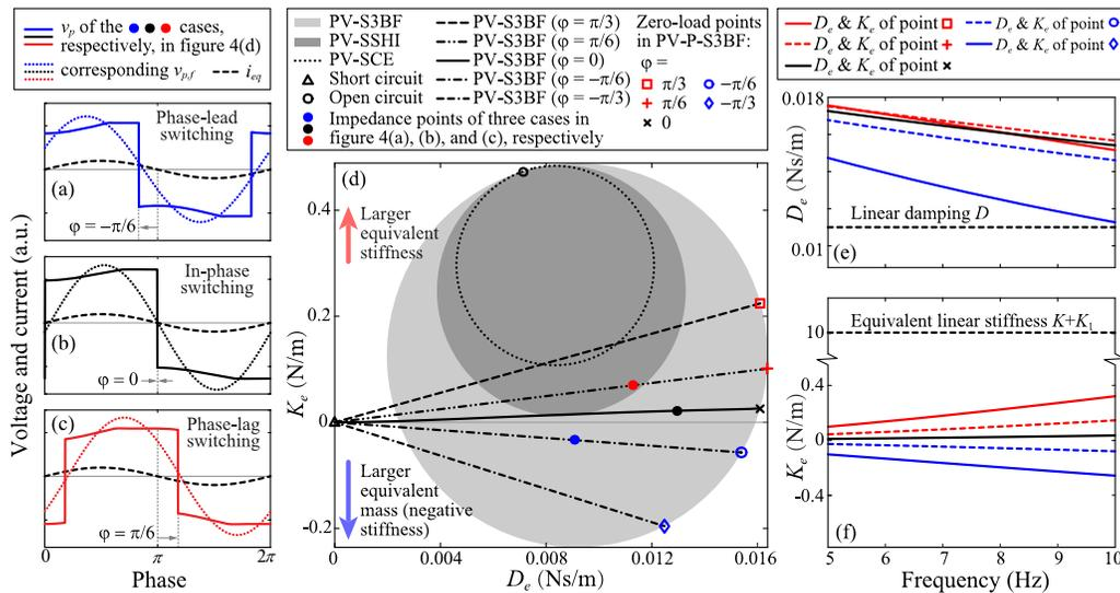
FIG. 4. Features of the PV-S3BF interface circuit. (a)–(c) Operating voltage and current waveforms under different switch phase lead/lag. (d) Equivalent impedance ranges of different circuits at 8 Hz vibration. (e) and (f) Electrically induced damping  $D_e$  and stiffness/mass  $K_e$  under the zero-loading condition.
