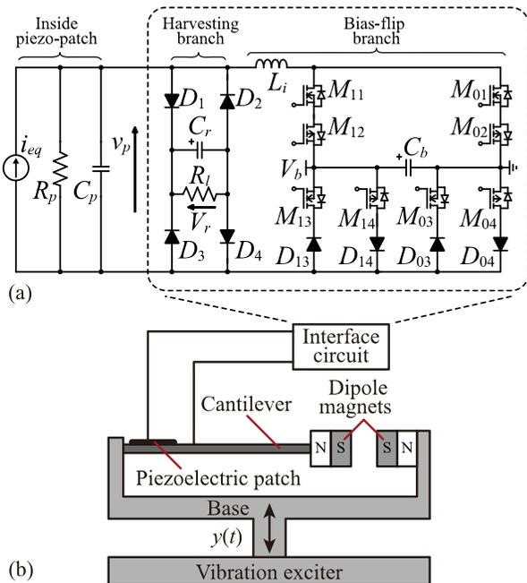
**FIG. 1.** Dual-effect broadband piezoelectric energy harvester, which is composed of (a) a PVSS interface circuit and (b) a nonlinear structure.
