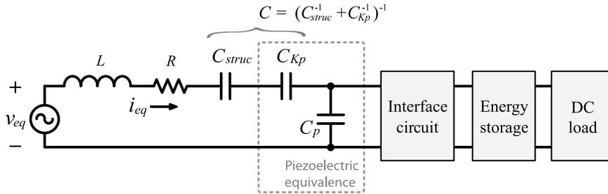
Figure 3. Equivalent circuit of a PEH device.
