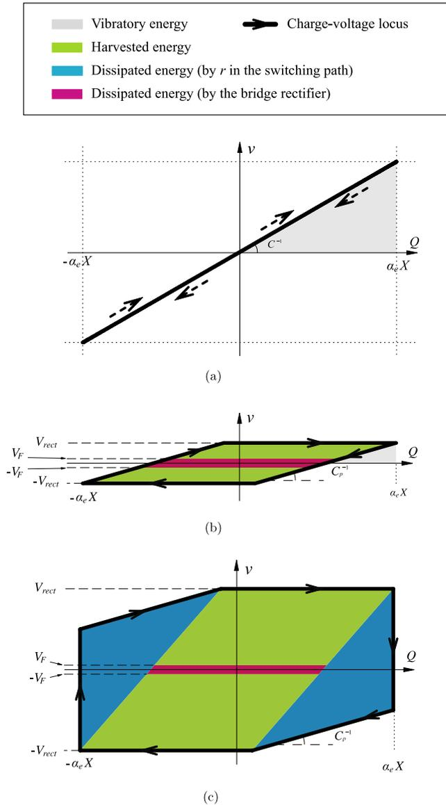
**Figure 8.** Charge–voltage diagrams. (a) Mechanical part. (b) Electrical part ( $\gamma = 1$ ,  $\tilde{V}_{rect} = 0.45$ ,  $\theta = 1.47$ ). (c) Electrical part ( $\gamma = -0.5$ ,  $\tilde{V}_{rect} = 1.8$ ,  $\theta = 1.47$ ).
