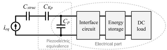
Figure 4. Equivalent circuit under constant displacement excitation.
