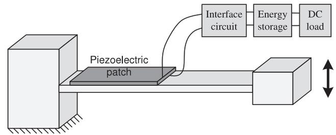
Figure 1. A typical cantilevered PEH device.
