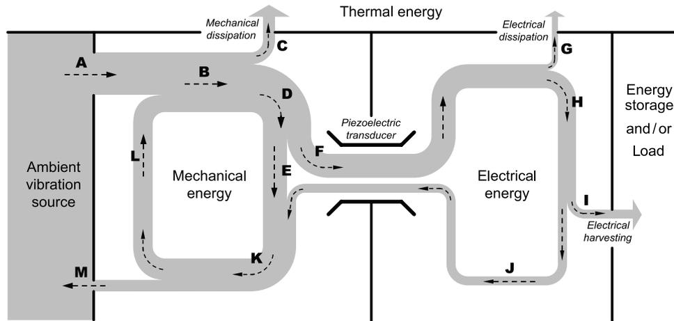
Figure 5. Energy flow chart in general PEH devices.
