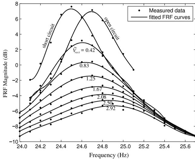
**Figure 11.** Frequency response functions under different electrical conditions.
