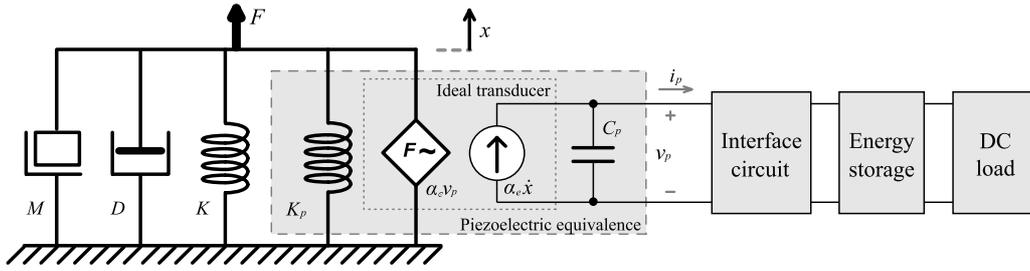
Figure 2. SDOF schematic representation of a PEH device.
