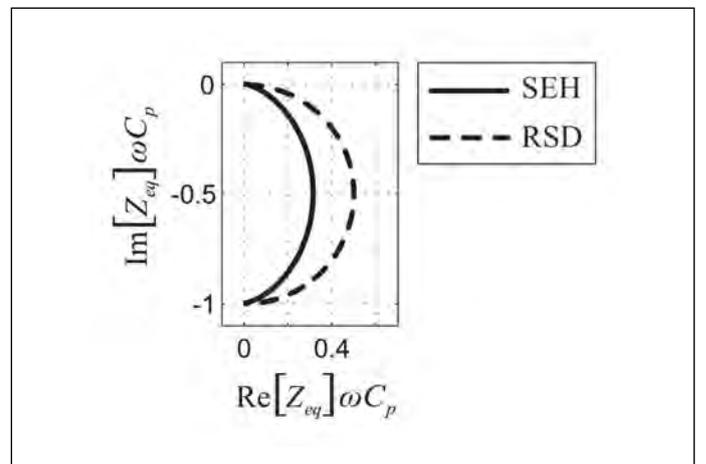
Figure 5 – Equivalent Impedance of SEH and RSD
