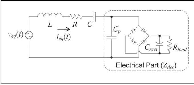
Figure 3 – Equivalent Circuit of a Base Excited PEH Device
