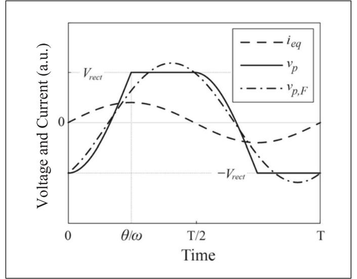
Figure 4 – Characteristic Voltage and Current Waveforms in SEH
