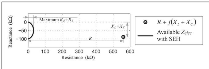
Figure 11 – Equivalent Impedance of the Mechanical and Electrical Parts
