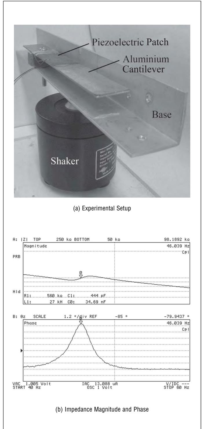
Figure 9 – Experimental Setup and Measured Impedance
