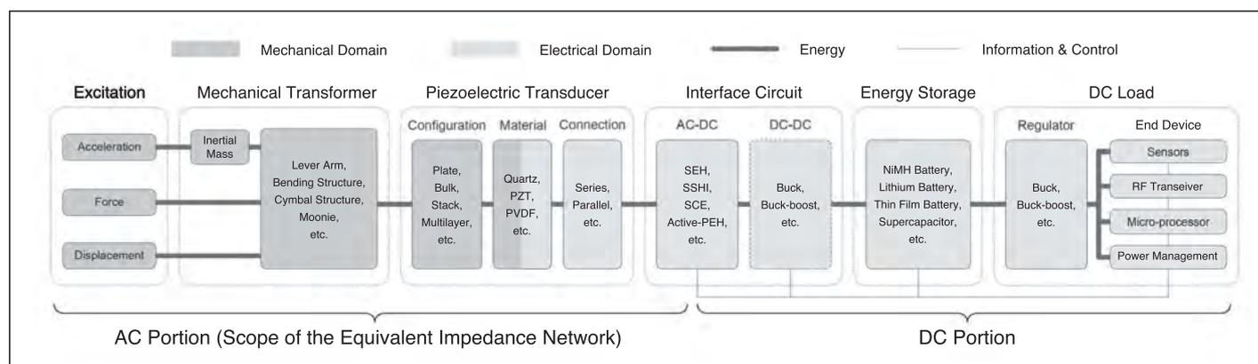
Figure 1 – Block Diagram of a PEH System
