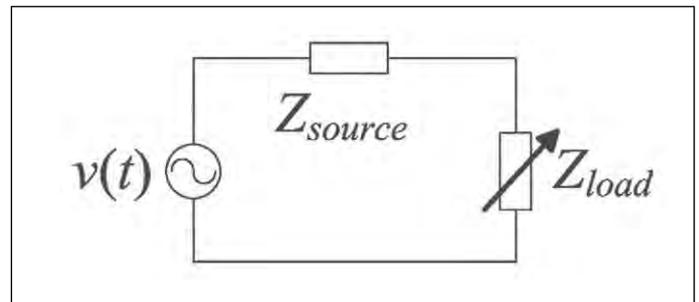
Figure 8 – Conventional Series Impedance Network with a Voltage Source
