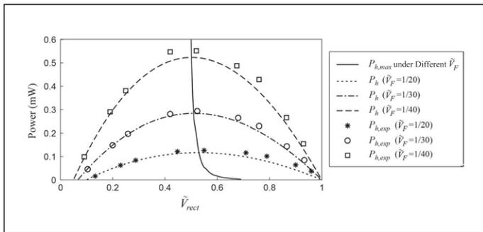
Figure 10 – Harvested Power as Functions of Rectified Voltage  $\tilde{V}_{rect}$
