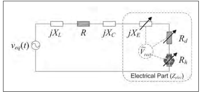
Figure 7 – Equivalent Impedance Network of a Base Excited PEH Device
