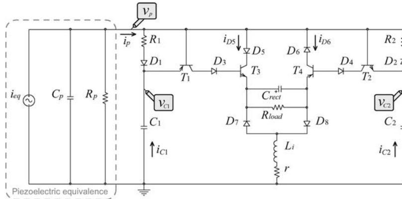
Fig. 4. Modified SP-SSHI interface circuit.
