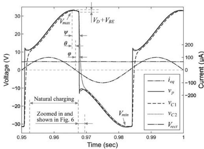
Fig. 5. Simulation waveforms in the modified SP-SSHI.
