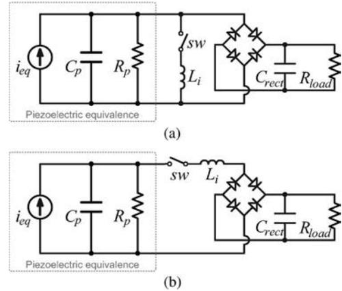
Fig. 2. Equivalent circuits of two SSHI treatments. (a) P-SSHI. (b) S-SSHI.
