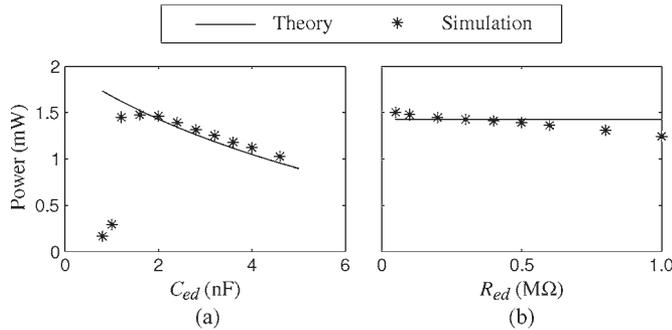
Fig. 9. Sensitivities of the harvested power. (a) Over the capacitance in the envelop detectors, i.e.,  $C_{ed}$  ( $R_{ed} = 200$  kΩ,  $V_{OC,org} = 25$  V,  $V_{DC} = 10$  V). (b) over the resistance in the envelop detectors, i.e.,  $R_{ed}$  ( $C_{ed} = 2$  nF,  $V_{OC,org} = 25$  V,  $V_{DC} = 10$  V).
