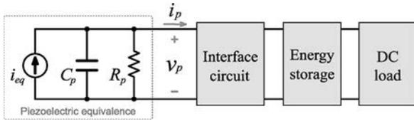
Fig. 1. Equivalent circuit of a PEH device.
