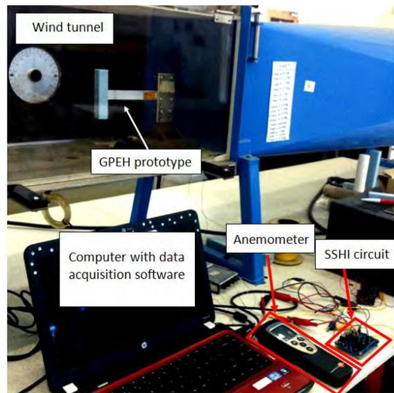
Figure 8. Overall experiment setup in the wind tunnel
