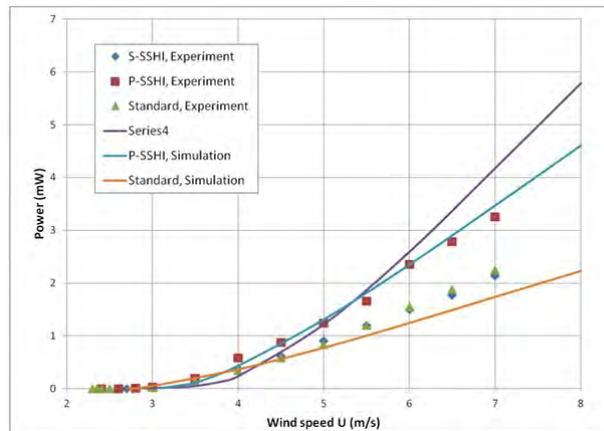
Figure 10. Measured and predicted power versus wind speed, with  $R_L=412k\Omega$  for the standard circuit,  $R_L=375k\Omega$  for S-SSHI and  $R_L=445k\Omega$  for P-SSHI.
