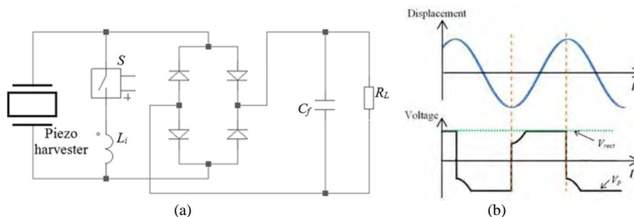
Figure 4. (a) P-SSHI interface circuit and (b) waveforms of voltage and tip displacement
