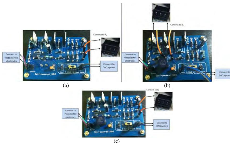
Figure 7. Hardware configuration for (a) the standard circuit (b) self-powered S-SSHI circuit and (c) self-powered P-SSHI circuit.
