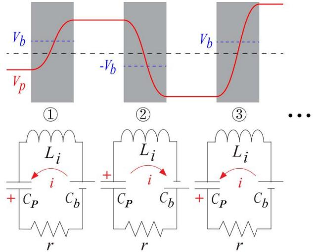
**FIGURE 2: VIBRATION EXCITING AT UPSTAIRS AND ITS EQUIVALENT CIRCUIT. ODD NUMBERS DENOTE POSITIVE CHARGING WHILE EVEN NUMBERS REPRESENT THE NEGATIVE CHARGING PROCESS. THREE CONSECUTIVE CHARGING PROCESSES ARE SHOWN HERE, MORE ACTIONS CAN BE ADDED AT EACH PIEZOELECTRIC VOLTAGE EXTREME.**
