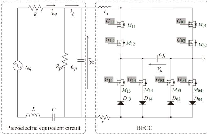
**FIGURE 1: PIEZOELECTRIC ENERGY HARVESTER WITH THE BECC CIRCUIT.**
