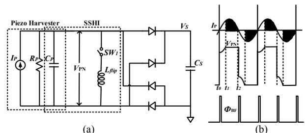
Fig. 1. SSHI circuit for PEH and the associated waveforms, (a) structure diagram of SSHI circuit, and (b) working waveforms.
