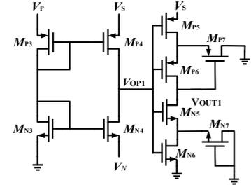
Fig. 3. The proposed self-biased common-gate comparator with unbalanced Schmitt trigger.
