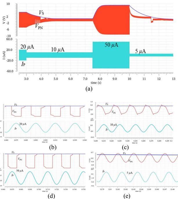
Fig. 6. Simulated transient characteristic of PEH interface circuit under different input currents, (a) transient characteristic under current variation, (b) 20- $\mu\text{A}$  input current, (c) 10- $\mu\text{A}$  input current, (d) 50- $\mu\text{A}$  input current, and (e) 5- $\mu\text{A}$  input current.
