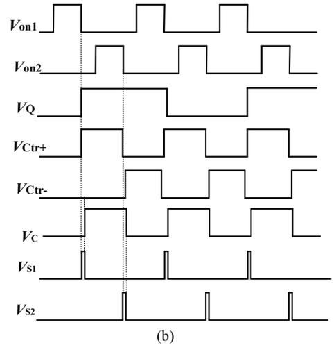
Fig. 4. (a) Switching signal control circuit for SSHI and (b) the associated working phases.
