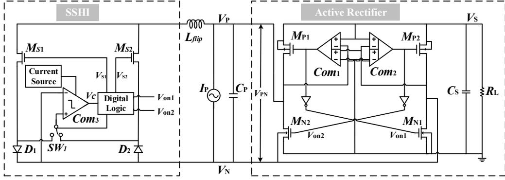
Fig. 2. Simplified diagram of the proposed self-powered SSHI interface circuit.
