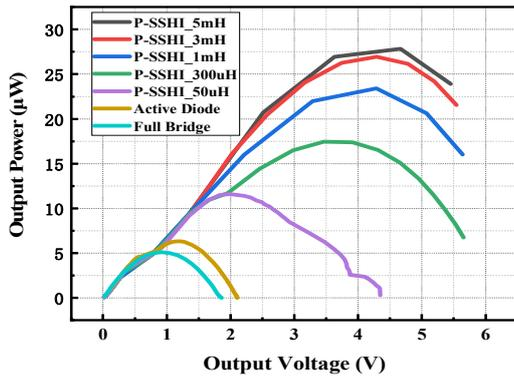
Fig. 7. Simulation of output power vs output voltage of SSHI and FB rectifier circuits
