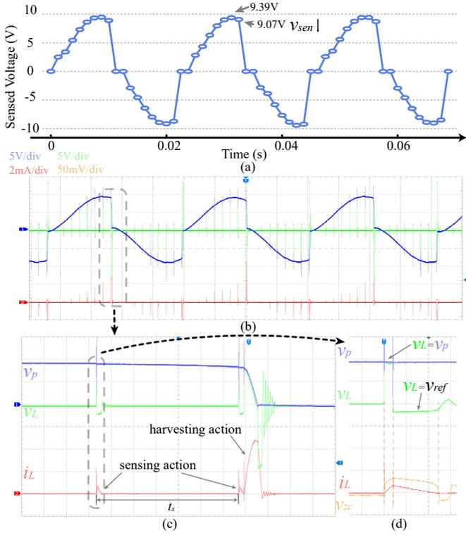
Fig. 5. SS-SECE waveform. (a) The sensed voltage  $v_p$  by the self-sensing solution; (b) Oscilloscope waveform. (c) The zoom-in view showing the current and voltage during sensing and harvesting instants. (d) A further zoom-in view of the sensing instants.
