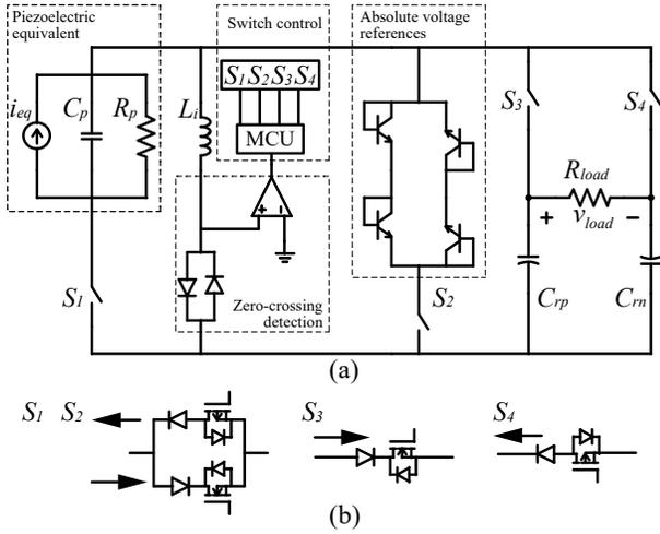
Fig. 2. Self-sensing SECE proposed in this paper. (a) Circuit topology. (b) Switch implementations.
