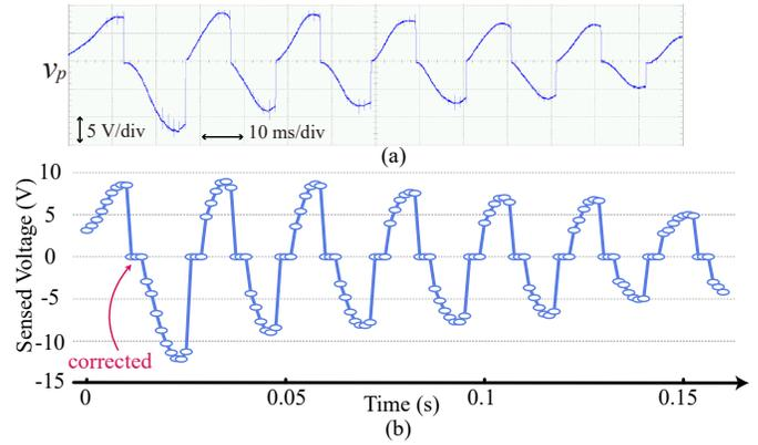
Fig. 7. Operating waveform under a shock vibration. (a) Oscilloscope measurement. (b) Measurement result with SS-SECE.
