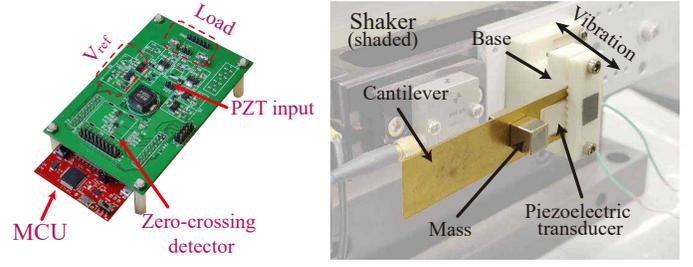
Fig. 4. SS-SECE PCB prototype and piezoelectric structure.
