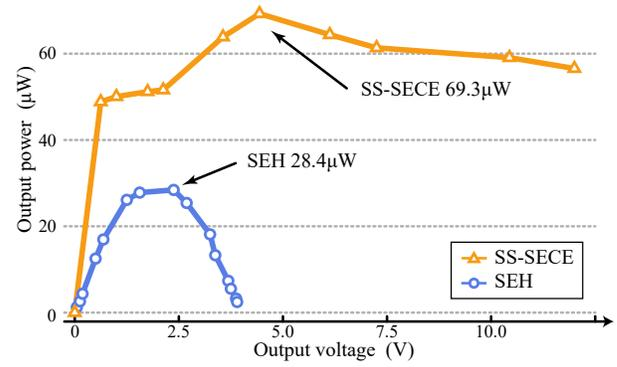
Fig. 6. Harvested power comparison.
