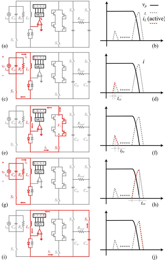
Fig. 3. The working phases and waveform of self-sensing SECE in the positive  $v_p$  half cycle. (a) and (b) Open-circuit phase. (c) and (d) Charge extraction phase in sensing mode. (e) and (f) Freewheeling phase in sensing mode. (g) and (h) Charge extraction phase in harvesting mode. (i) and (j) Freewheeling phase in harvesting mode.
