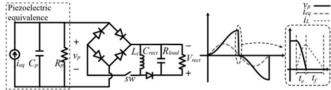
Fig. 1. Conventional SECE circuit topology and waveform.
