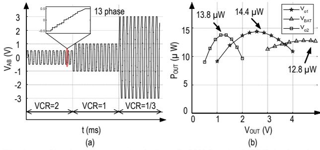
Fig. 8. (a) Simulated  $V_{AB}$  with 13-phase P-SSHC under MPPT (b) Simulated  $P_{OUT}$  at different outputs.
