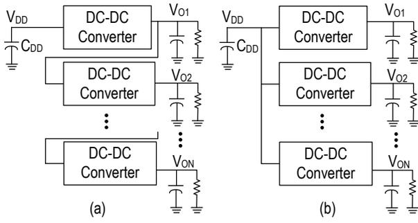
Fig. 5. Two structures of multi-output DC-DC converters. (a) Series structure. (b) Parallel structure.
