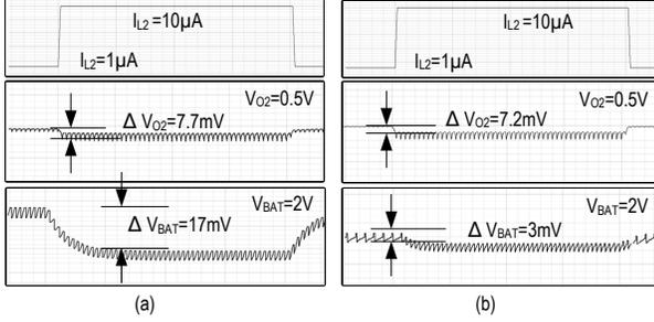
Fig. 9. Cross regulation of multi-output SC DC-DC converters with series and parallel structures. (a) Series structure (b) Parallel structure
