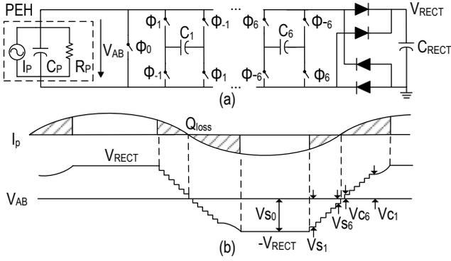
Fig. 2. P-SSHC rectifier with 6 SCs and associated waveforms
