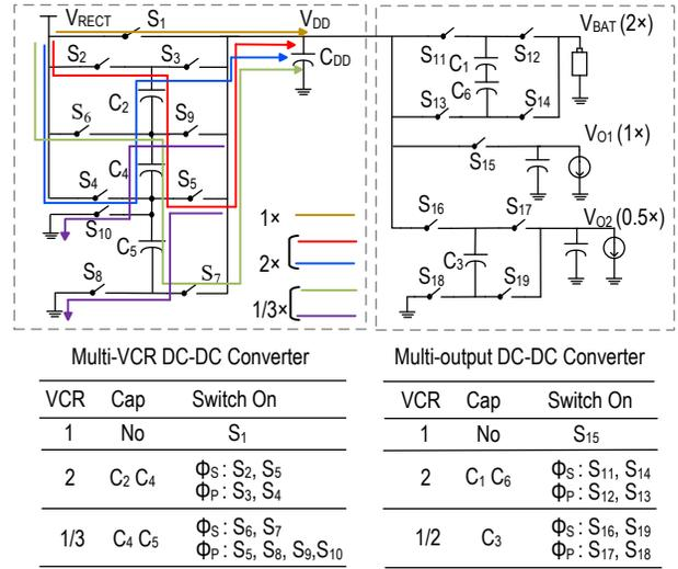
Fig. 4. Circuit of SC DC-DC converters
