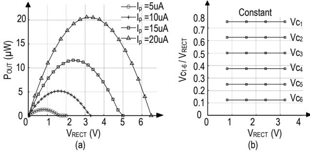
Fig. 3. (a) Simulated  $P_{OUT}$  with respect to  $V_{RECT}$  at different excitation. (b) Ratios of voltages on flying capacitors  $V_{C_i}$  over rectifier voltage  $V_{RECT}$ .
