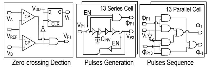
Fig. 6. Controller circuit of P-SSHC rectifier
