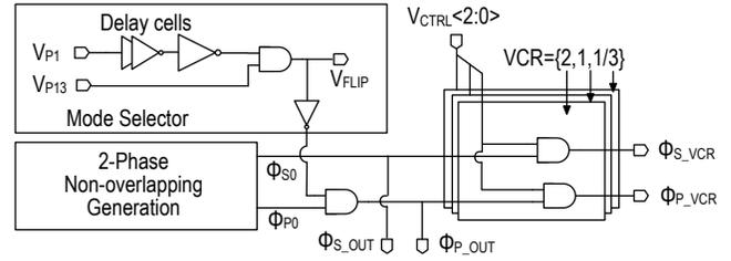
Fig. 7. The circuit of SC DC-DC drivers
