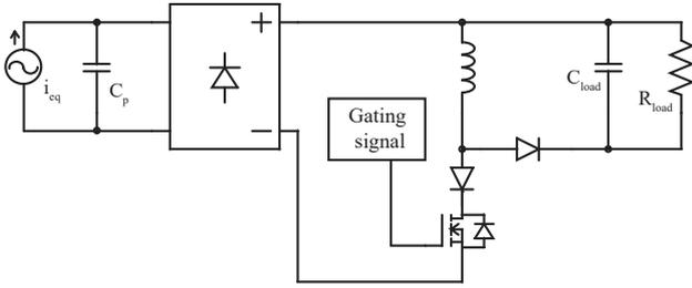
Fig. 2. SECE interface circuit
