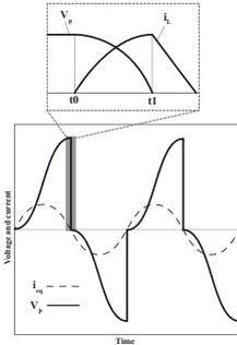
Fig. 3. Voltage and current waveform of SECE circuit
