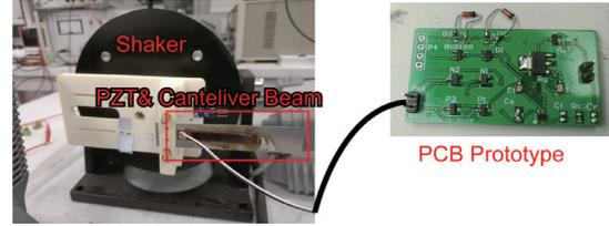
Fig. 10. Shaker, cantilever beam and PCB prototype used in experiments. The inductor is externally connected.
