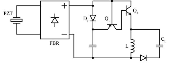
Fig. 9. Conventional self-powered SECE interface circuit based on peak detection [13]
