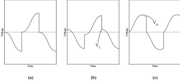
Fig. 8. Incomplete Charge Extraction. (a) Ideal SECE waveform with no incomplete charge extraction. (b) Incomplete charge extraction due to residual charge. (c) Incomplete charge extraction due to peak detection delay
