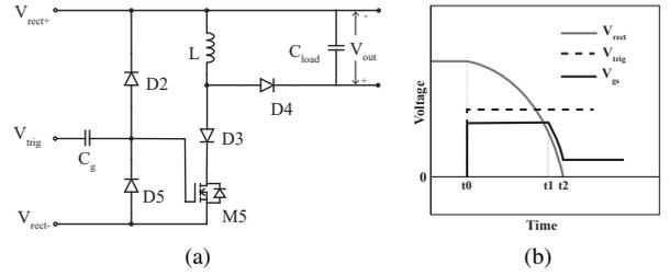
Fig. 7. Passive zero crossing detection and turning off. (a) schematic. (b). voltage waveform of  $V_{gs}$  of M5,  $V_{rect}$  and  $V_{trig}$
