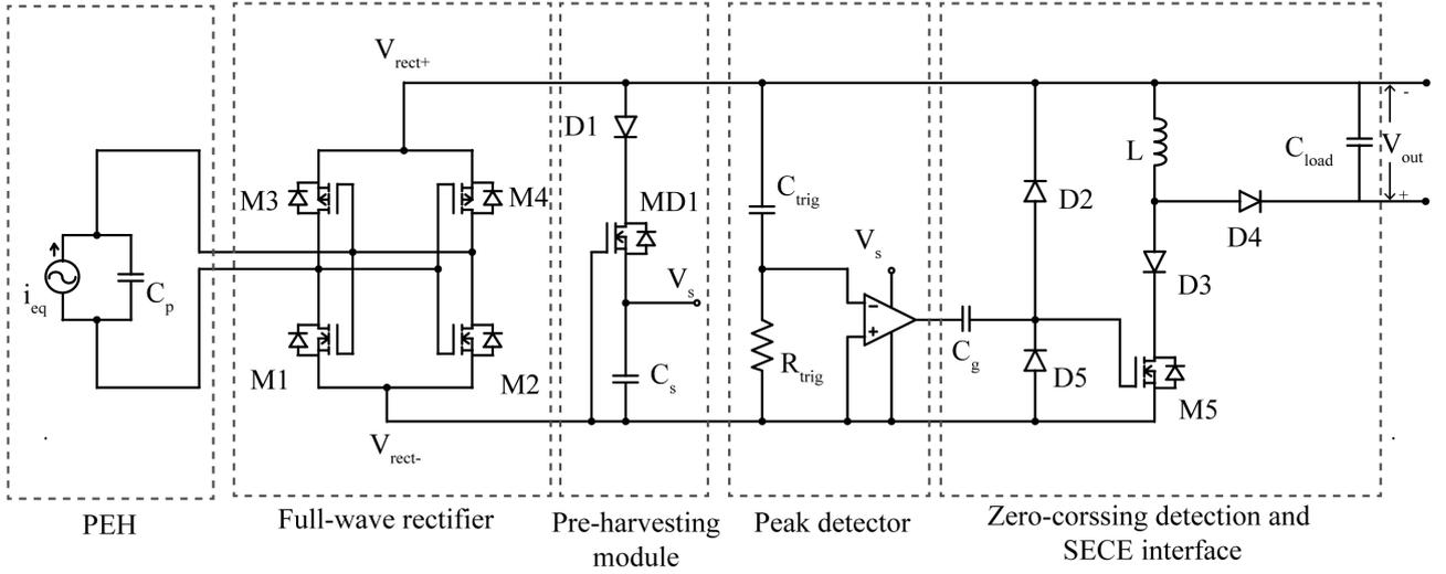
Fig. 1. Overview of proposed interface circuit.
