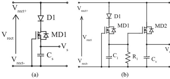
Fig. 5. Pre-harvesting circuit. (a) One stage pre-harvesting circuit. (b) Cascoded pre-harvesting circuit.
