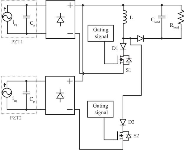
Fig. 4. SECE circuit for PEH array with two PEHs
