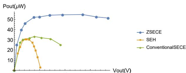
Fig. 11. Output power of ZSECE, Full bridge rectifier (SEH) and conventional self-powered SECE in Fig. 9
