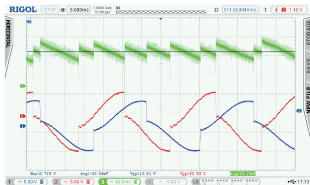
Fig. 12. Voltage waveform of two PEHs (red and blue) and output voltage (green)
