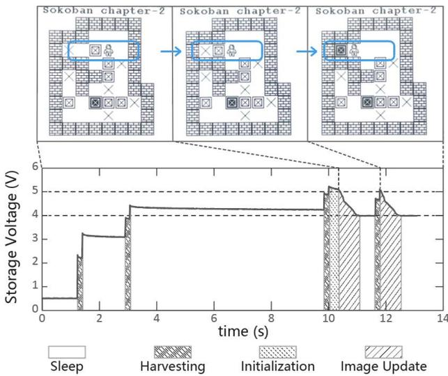
Figure 3: Experimental work cycle.
