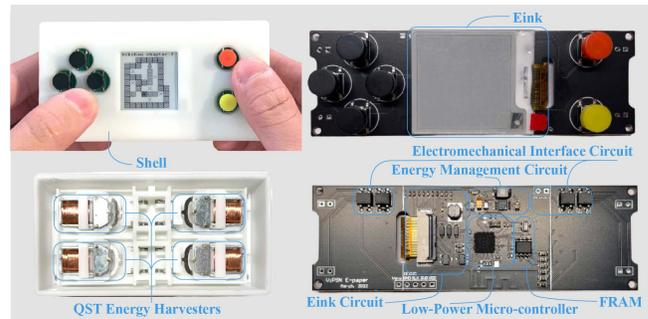
Figure 1: Hardware Prototype.
