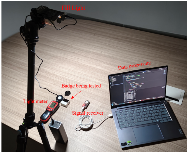
Figure 3: Experiment setup of single badge evaluation.
