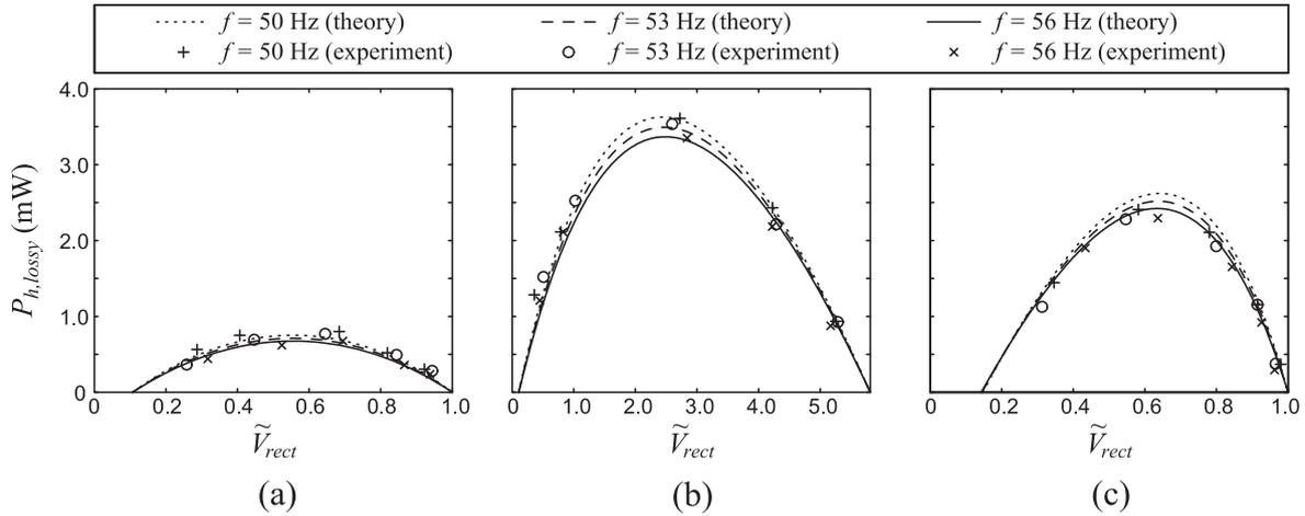
**Figure 5.** Results in experiment #1 (constant  $\dot{X}$  and infinite  $R_{p,ex}$ ). (a) SEH. (b) P-SSHI. (c) S-SSHI.
