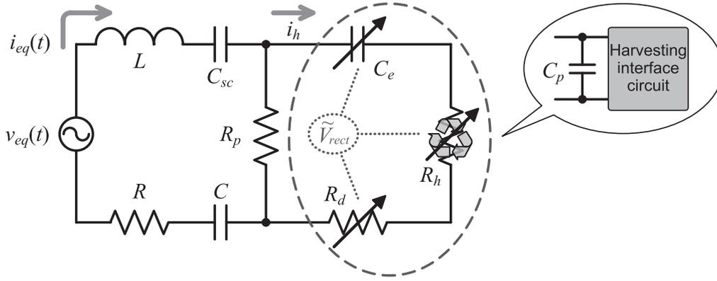
Figure 1. Equivalent impedance network of a PEH system.
