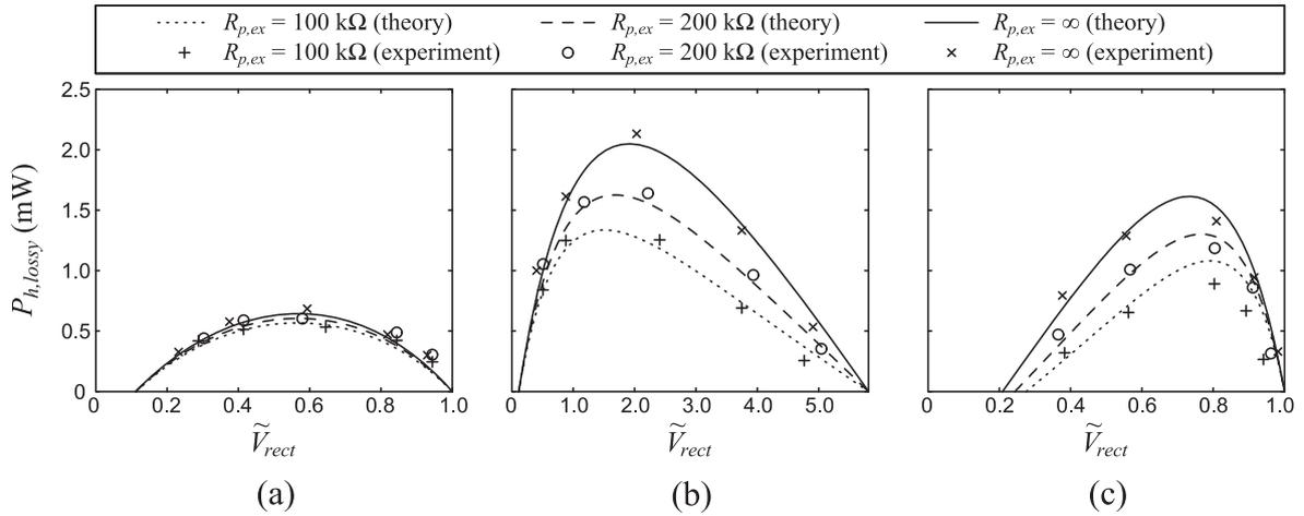
**Figure 8.** Results in experiment #4 (constant  $\ddot{Y}_{ex}$  and  $f$ ). (a) SEH. (b) P-SSHI. (c) S-SSHI.
