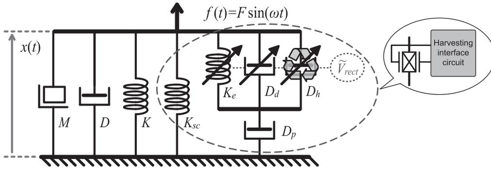
Figure 2. Equivalent mechanical schematics of a PEH system.
