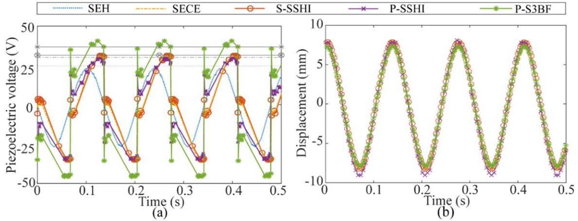
**Figure 6.** Experimental capture of piezoelectric voltage and mass displacement, (a) piezoelectric voltage history, the grey curves are analytically solved voltage amplitude, (b) displacement history.
