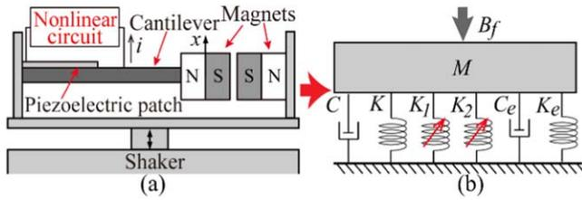
**Figure 1.** The nonlinear energy harvester with a nonlinear circuit (a) system overview; (b) equivalent lumped parameter model.
