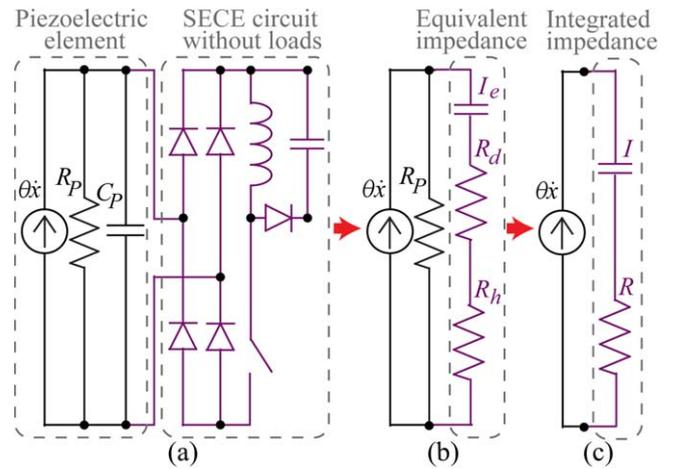
**Figure 2.** Equivalent circuit model (a) equivalent piezoelectric element connected with SECE without loads, (b) equivalent impedance, (c) integrated impedance.
