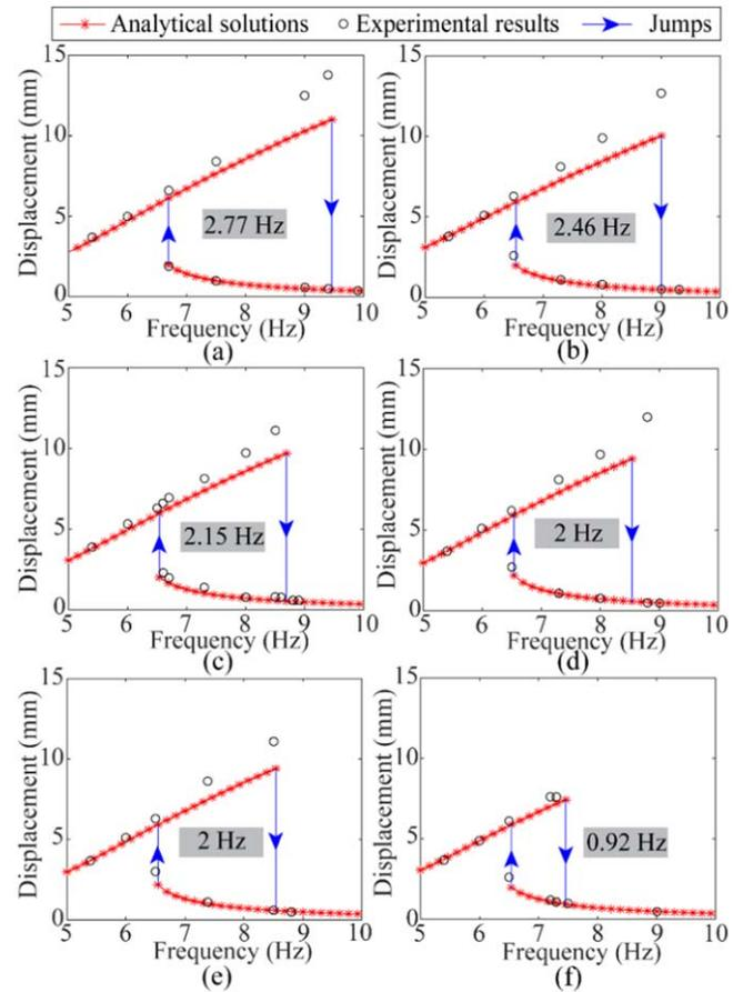
**Figure 3.** Frequency response of the monostable transformer connected with different nonlinear circuits. Red stars denote analytical solutions, while experimental results are marked by circles. The blue arrows define the jumps and hysteresis region size is highlighted by shading. (a) Pure mechanical structure, (b) SEH, (c) SECE, (d) S-SSHI, (e) P-SSHI, (f) P-S3BF.
