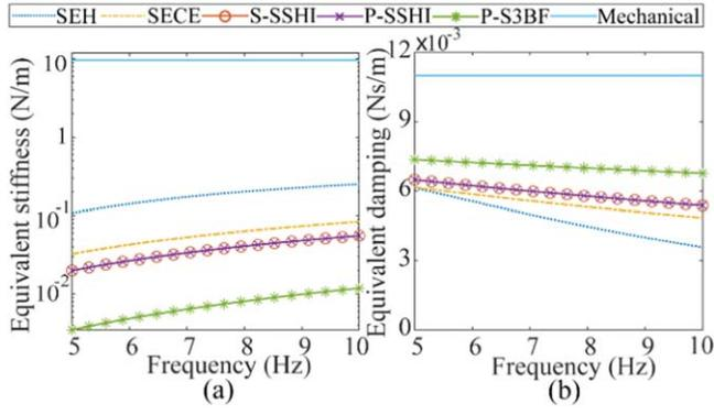
**Figure 4.** The circuit-induced stiffness and damping compared with mechanical stiffness and damping. (a) equivalent stiffness, (b) equivalent damping
